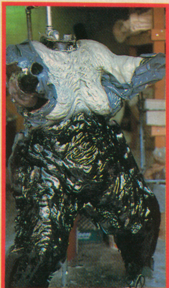
PHOTO 8: Black gel-coat resin is used for the first layer. The color makes troublesome bubbles easier to spot. I brought in fiberglass expert Don (Cocoon) Pennington for the job, and he fabricated a pristine mold.
