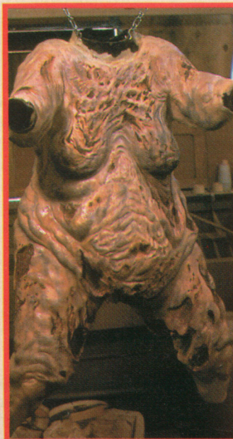
PHOTO 7: Henrietta's bloated plastilina body is done. In preparation for the fiberglass mold, we spray the clay with clear acrylic and several coats of PVA (a standard release for fiberglass).
